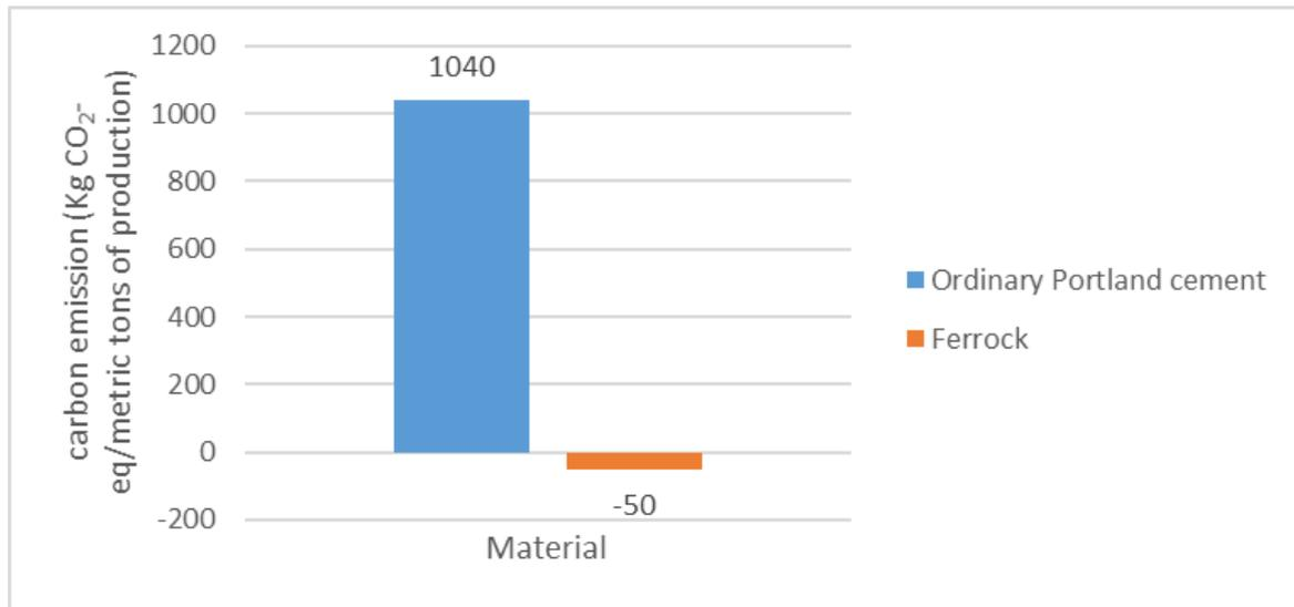
Figure 4. Carbon emission of Ferrock and OPC.
