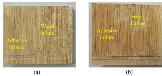
Figure 15. Surface area of specimen after block shear test: (a) bonded with polyvinyl acetate and (b) bonded with one-component polyurethane.
