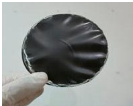
Figure 2. Photograph image of the as-cast composite film.
