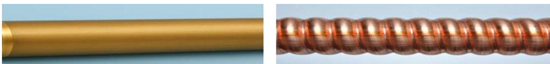
Figure 2. Inner pipes of the experimental DPHE setup: (a) smooth pipe, (b) circumferentially ribbed pipe.
