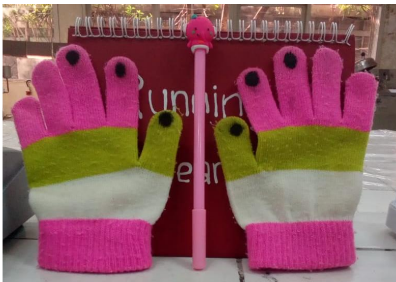
Figure 5. The right glove is graphite paste with polyacrylate and the left glove is graphite paste without polyacrylate
