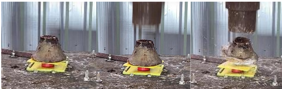
Figure 20. Progressive damage of the conical specimen during impact loading.
