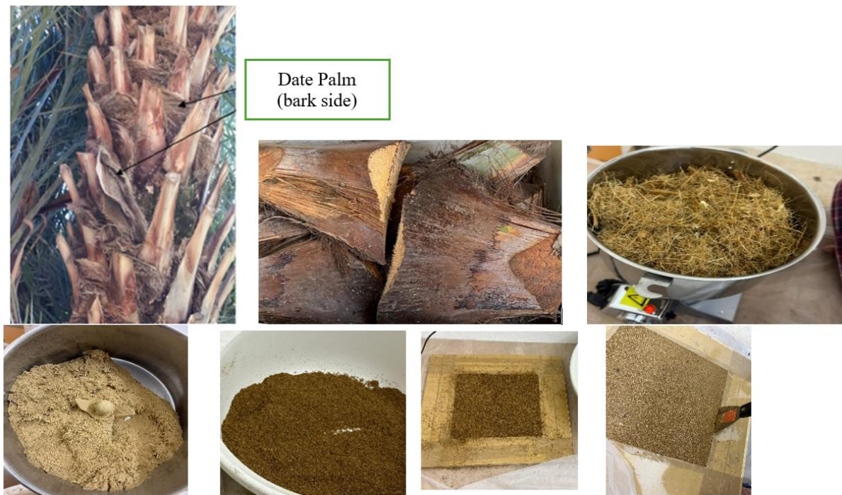
Figure 1. Preparation of date palm trunk bark powder for composite fabrication.
