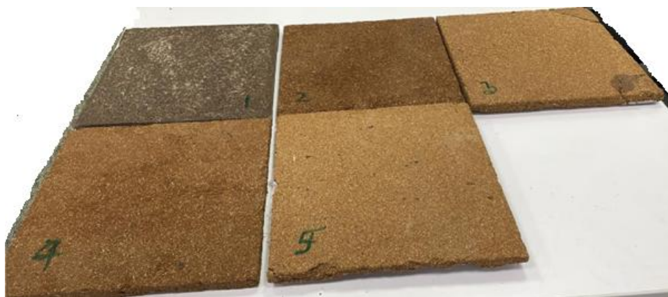
Figure 3. Fabricated epoxy/date palm trunk bark powder composite specimens with different filler loadings.
